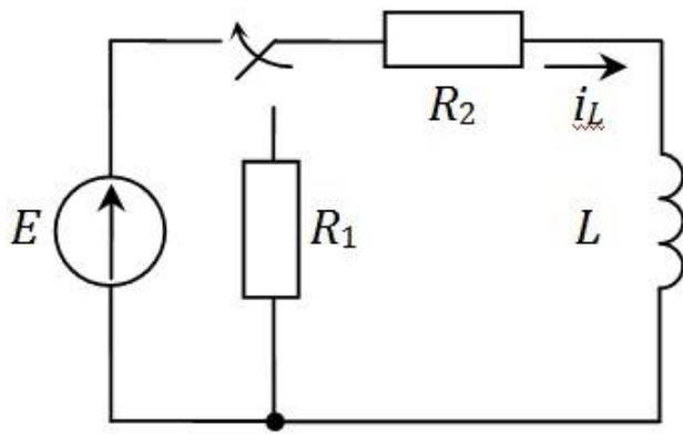
$$\tau = L \frac{R_1 + R_2}{R_1 R_2}$$
