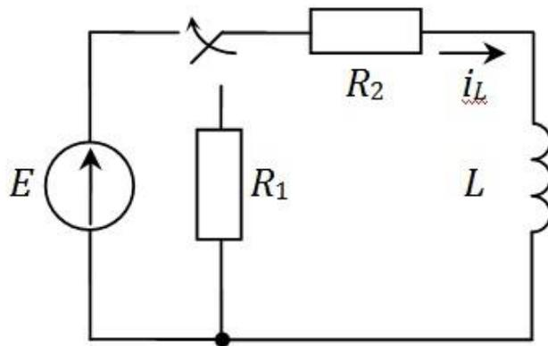
$$\tau = L \frac{R_1 + R_2}{R_1 R_2}$$
